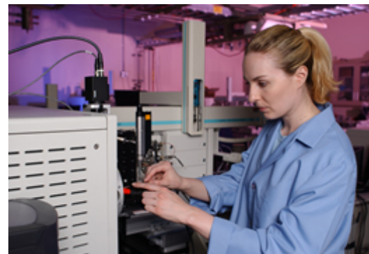
A PNNL scientist uses a ThermoFinnigan LTQ mass spectrometer to identify peptides from living organisms such as Salmonella and Orthopox viruses
